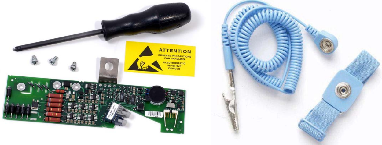
Fig. 2 ESD screwdriver and ESD wrist strap
